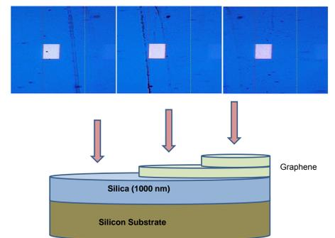
Figure 4: (top) Photos of the measurement region, left - substrate; middle - 1 sheet and right - 2 sheets. (bottom) - Sample model used for the ellipsometry data analyses.
