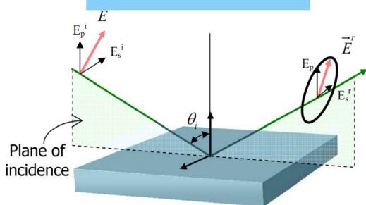
Figure 1: Incident linearly polarized light emerges from the reflection with elliptical polarization.
