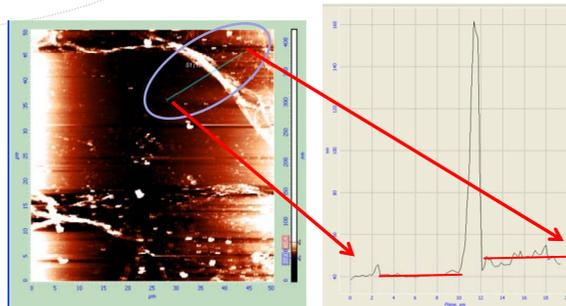
Figure 2: AFM mapping and profile along the substrate-graphene edge.
