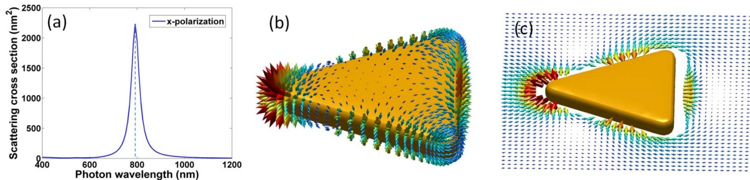
**Figure 4.4.:** (a) Scattering cross section of a gold nanotriangle ( $55 \times 50 \times 8 \text{ nm}$ ,  $n_b = 1.34$ ). The panels (b) and (c) show the electric field at the resonance energy of  $792 \text{ nm}$  at the particle surface and on the outside, respectively. (Also see Fig. 3.7.)
