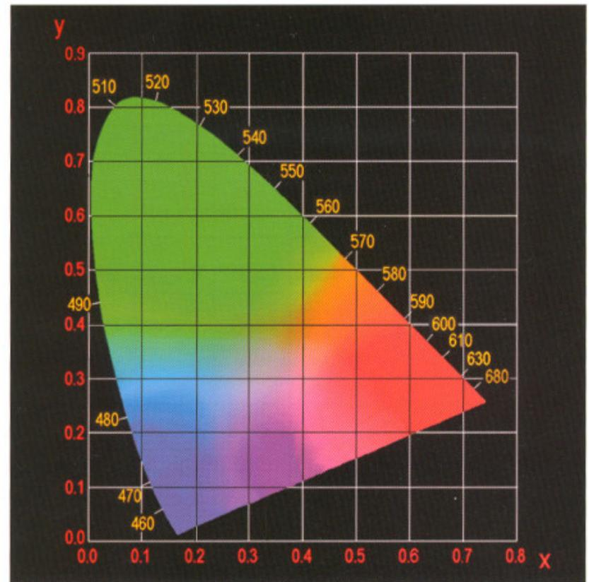
Figure 4.7 Color chromaticity  $x - y$  diagram for a 2-deg field (CIE 1931).
