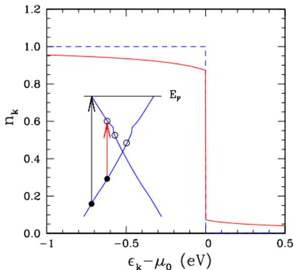
The probability of occupation of a state  $\mathbf{k}$ ,  $n_{\mathbf{k}} = \int_{-\infty}^{\infty} f(\omega) A(\mathbf{k}, \omega) d\omega$  for two cases: bare band (dashed blue curve) and with electron-phonon interaction included (solid red curve). The inset is a schematic which illustrates the renormalized energy bands filled to the Fermi level  $E_F$  with finite probability for some holes to exist below the Fermi level. Interband transitions are now possible for energies below  $2\mu$ .
