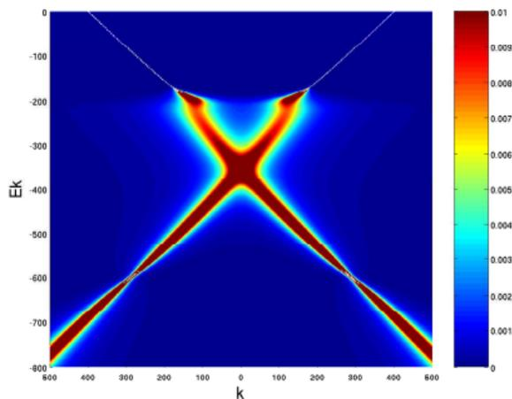
Color map (units of  $\text{meV}^{-1}$ ) of interacting dispersions  $E_k$  in units of  $\text{meV}$  as a function of  $\mathbf{k}$  in units of  $\text{meV}/(\hbar v_0)$ . The bare chemical potential  $\mu_0 = 400 \text{ meV}$  and a Lorentzian phonon spectrum with  $\omega_0 = 200 \text{ meV}$  were used. Broadening makes determination of  $\mu$  somewhat ambiguous.
