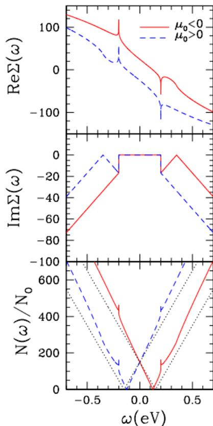
Real (top) and imaginary (middle) part of  $\Sigma(\omega)$  and DOS [first iteration]  $N(\omega)/N_0$  (bottom) (all in units of meV) as a function of  $\omega$  in eV for  $|\mu_0| = 150$  meV. Dashed is for  $\mu_0 > 0$  and solid is for  $\mu_0 < 0$ . The bare band DOS is indicated by the dotted curve.
