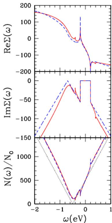
$\Sigma(\omega)$  and DOS have been self-consistently iterated and  $\mu_0 = 500 \text{ meV}$  which is greater than  $\omega_E$ . The red solid curves are for the iterated case and the blue dashed curves are for the initial uniterated results. The dotted curve is the bare density of states. All quantities on the y-axis are in meV.
