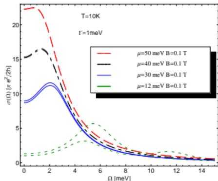
$\text{Re}\sigma_{xx}(\Omega)$  in units  $\pi e^2/2h$  for  $B = 0.1 \text{ T}$ ,  $T = 10 \text{ K}$ , and scattering rate  $\Gamma = 1 \text{ meV}$ . For green line  $\mu$  is getting close to  $E_1 = 11.5 \text{ meV}$ .
