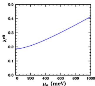
The mass renormalization parameter  $\lambda^{\text{eff}}$  at the Fermi level as a function of bare chemical potential  $\mu_0$ . At least 20 % renormalization of  $v_0$ .
