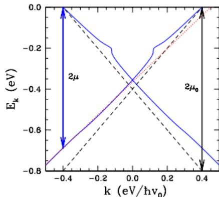
Renormalized energies (solid blue curves)  $E_k$  as a function of  $k$  in units of  $\text{eV}/(\hbar v_0)$  for  $\mu_0 = 400 \text{ meV}$ . Twice the bare  $2\mu_0$  and dressed  $2\mu$  chemical potential are indicated by vertical arrows.
