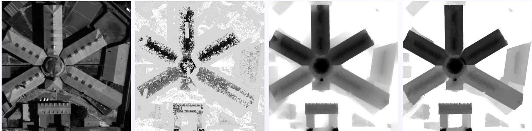
Figure 17: Disparity interpolation in an urban digital elevation model. reference image, incomplete data set (30% of the image), interpolation with the minimal surface interpolation (RMSE 0.239) and with the proposed algorithm (RMSE 0.190).
