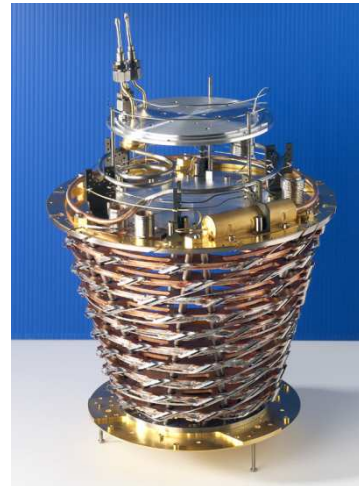
Heat exchanger of the dilution cooler (1.6 – 0.1 K)
