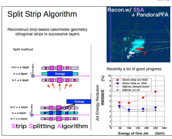
Novel approach: a very compact, tungstene-Silicium electromagnetic calorimeter
