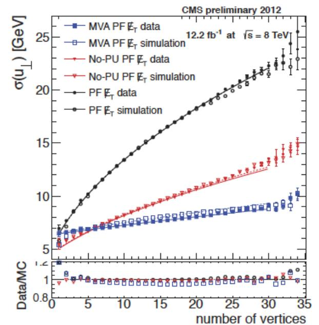
Figure 19: Parallel (top) and perpendicular (bottom) resolution as a function of the number of reconstructed vertices for PF  $\vec{E}_T$ , No-PU PF  $\vec{E}_T$ , and MVA PF  $\vec{E}_T$  in  $Z \rightarrow \mu^+\mu^-$  (left) and  $Z \rightarrow e^+e^-$  (right) events.
