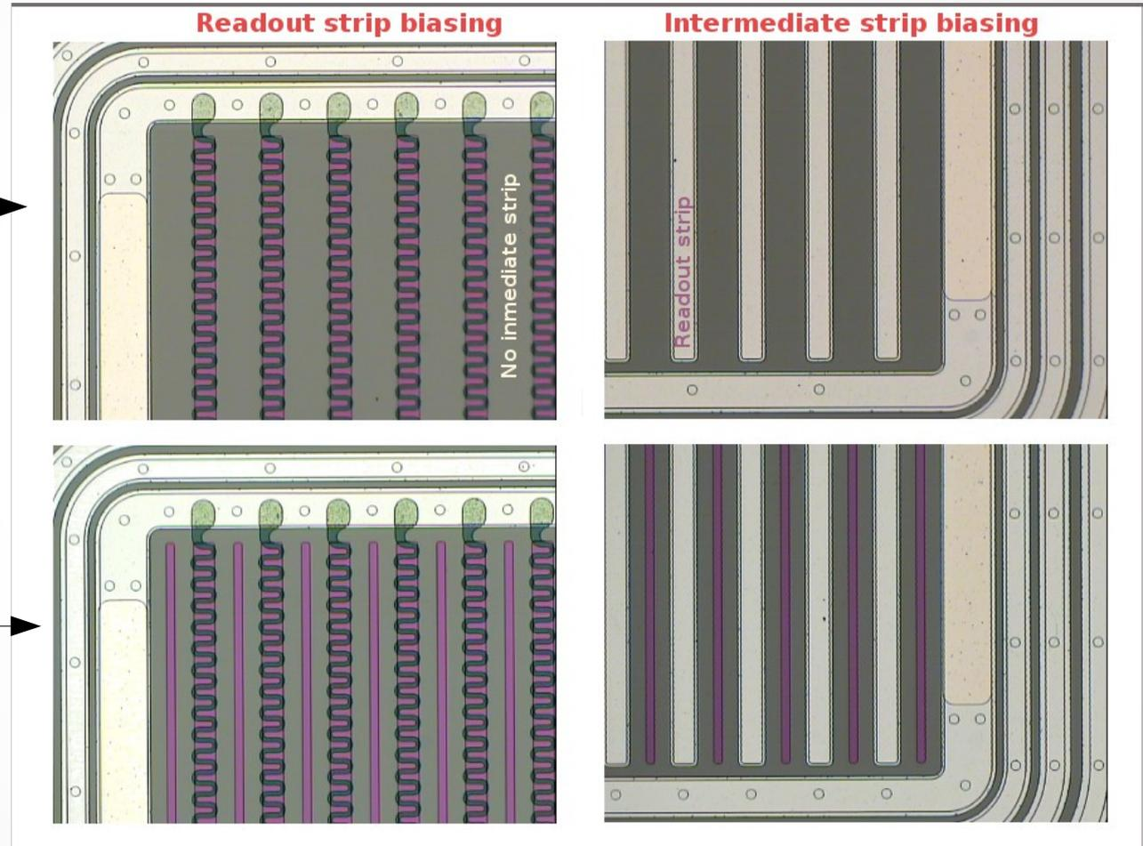
Intermediate strips are left *unbiased*, so they are called *floating intermediate strips*.
