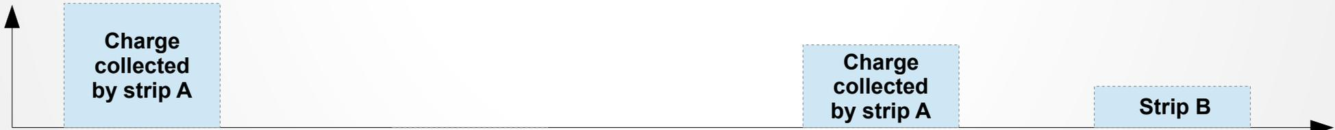
As the distribution charge function of the interstrip-free model is a step function, strip A collects all the charge created by the incoming particle in detector **M-14**.
