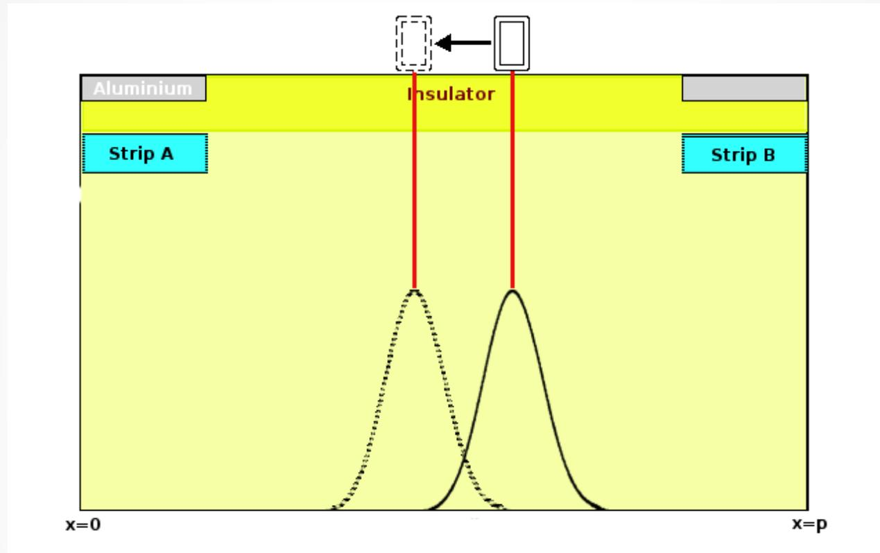
As the laser beam shape follows a gaussian distribution, when laser is centered in a position  $x$ , a small region is lightened. What is measured then is the convolution of the detector charge distribution function,  $q(x)$ , with the gaussian profile of the laser beam, given by:
