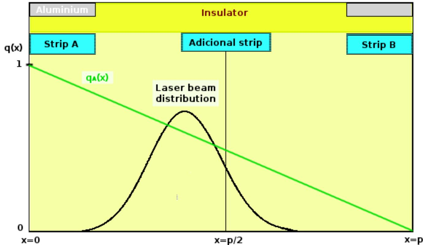
$q(x)$  is a linear function  $\longrightarrow$  It allows the use of weighting techniques
