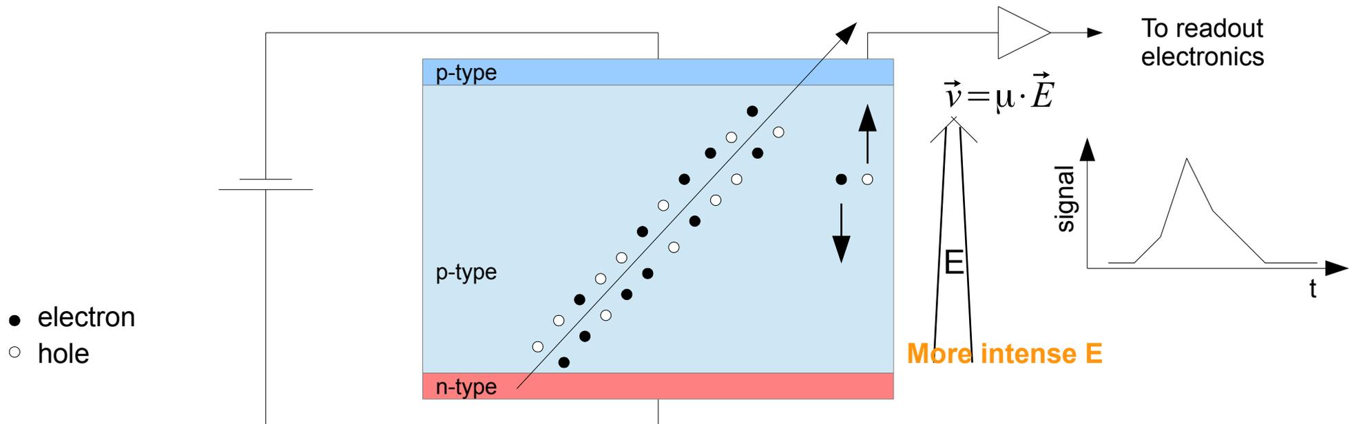
The electric field is more intense at the p-n junction (backplane) → As carriers velocity is:  $v = \mu E$  → carriers slow down as they approach the readout contact
