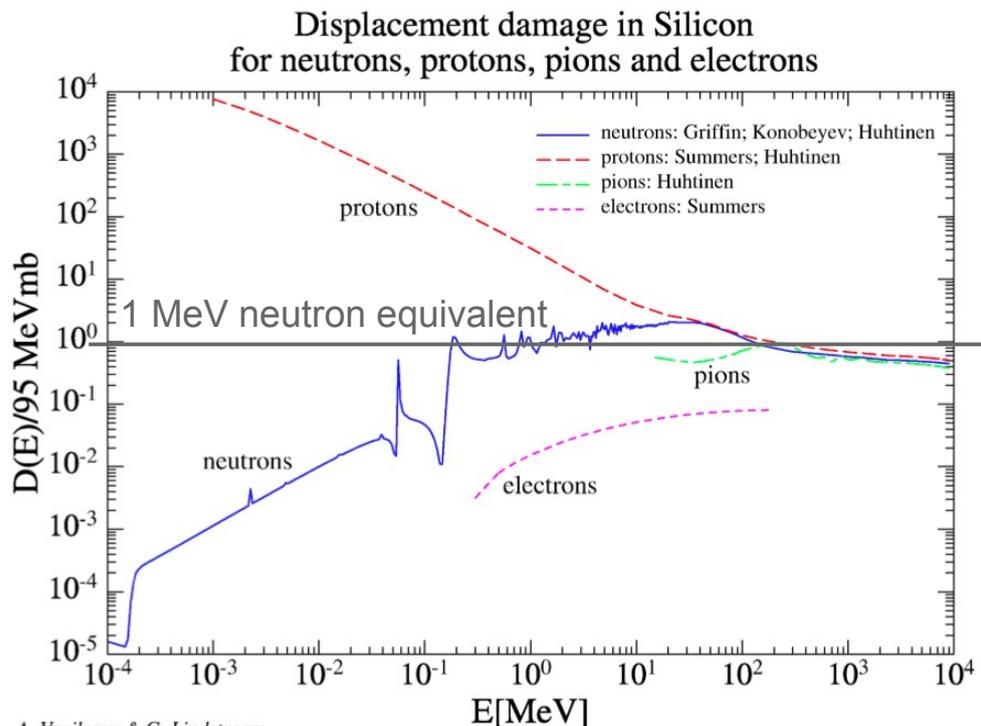
Damage hardness factor for different particles
