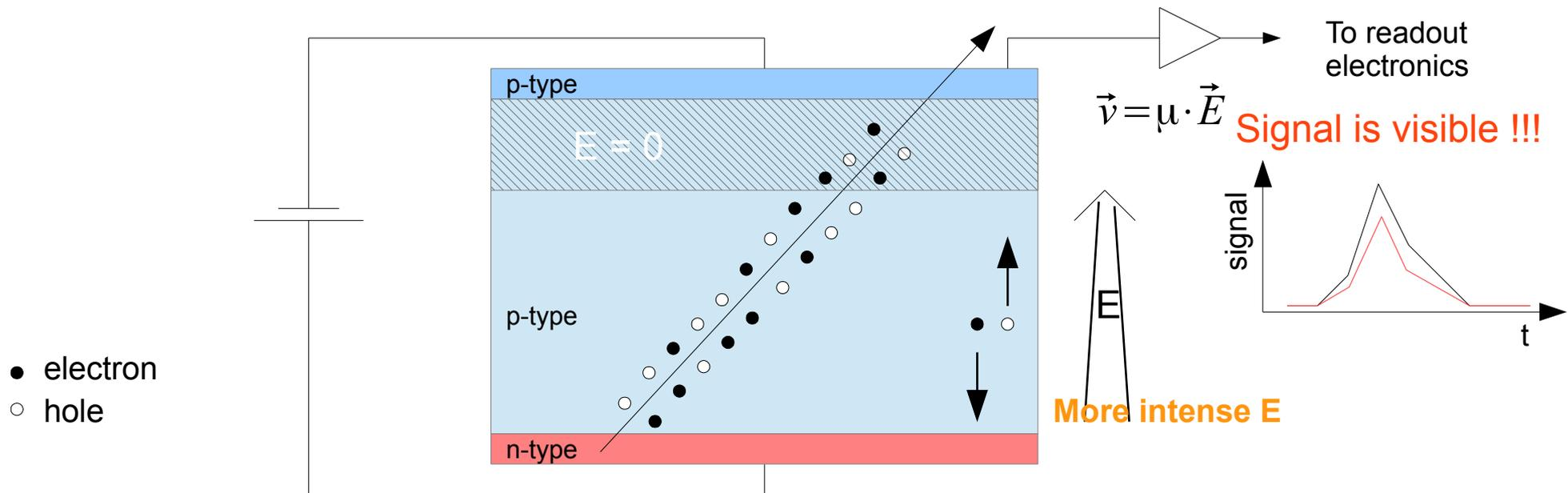
In spite of the  $E=0$  region near the readout channels signal is still visible because the charge carriers move in the depleted region → the current produces signal although spatial resolution degrades
