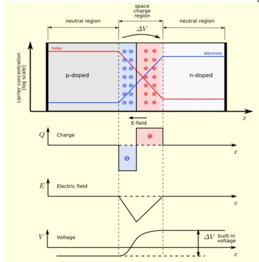
Still, thermal excitation creates e-h pairs in everywhere and of course in the depleted zone. The electric field there splits electrons and holes in opposite directions thus producing a **LEAKAGE CURRENT**
