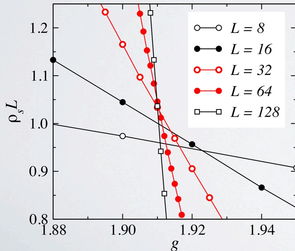
According to theory, spin stiffness at the critical point should scale according to ( $T=0$ )
