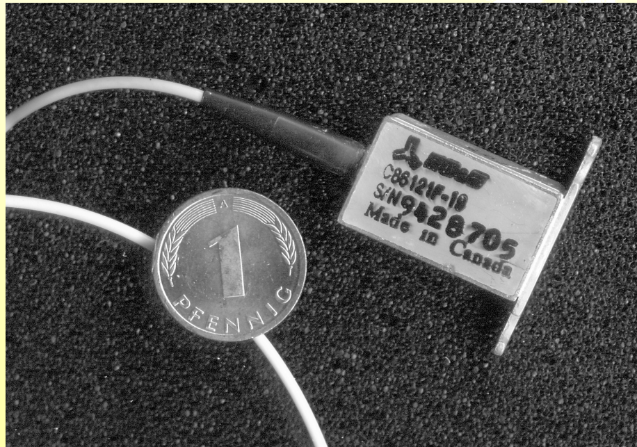
packaged laser diode with monitor, cooler, pigtail
