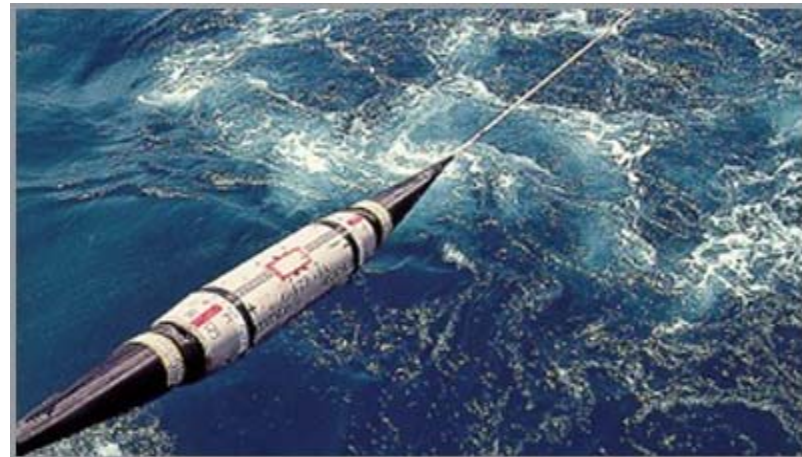
Repeaters based on Optical Signal (Undersea Cables)
