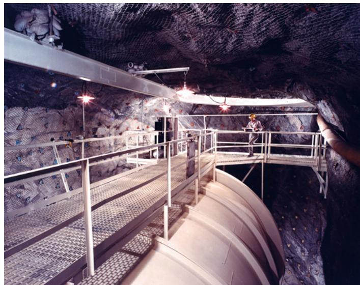
$n + ^{37}\text{Cl}$  makes  $^{37}\text{Ar}$  that decays back to  $^{37}\text{Cl}$  with a half-life of 35 days. Ray Davis used this to measure neutrinos from the sun. Basically get a big vat of  $\text{CCl}_4$ , put it 4850' deep in a gold mine, extract Argon atoms and count Ar decays.
