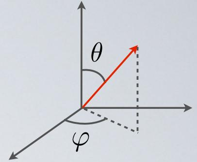
$$h_+(t, \theta, \varphi) = \frac{G}{r} \left[ \ddot{M}_{11}(\cos^2 \varphi - \sin^2 \varphi \cos^2 \theta) + \ddot{M}_{22}(\sin^2 \varphi - \cos^2 \varphi \cos^2 \theta) \right. \\ - \ddot{M}_{33} \sin^2 \theta - \ddot{M}_{12} \sin 2\varphi(1 + \cos^2 \theta) + \ddot{M}_{13} \sin \varphi \sin 2\theta \\ \left. + \ddot{M}_{23} \cos \varphi \sin 2\theta \right]$$
