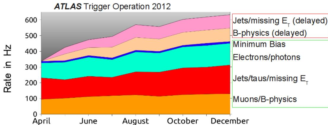
Both experiments have improved their DAQ and trigger systems for Run-2. Current DAQ Performance
