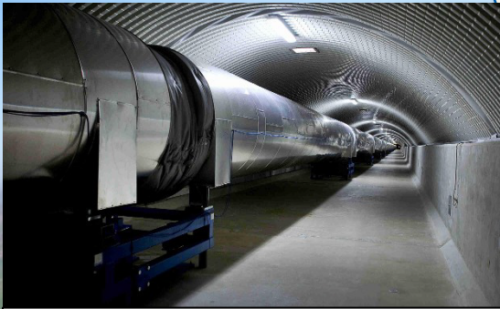
UHV to avoid pressure fluctuations
