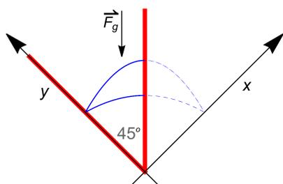
the mirrors are located around  $x = 0$  and  $x - y = 0$  and form a wedge with the angle  $45^\circ$
