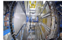
ATLAS gas detector based muon spectrometer, which covers a large area of the solid angle of a hadron field and measures the paths of the muons that pass through it to an accuracy of better than a tenth of a millimetre. (© CERN)
