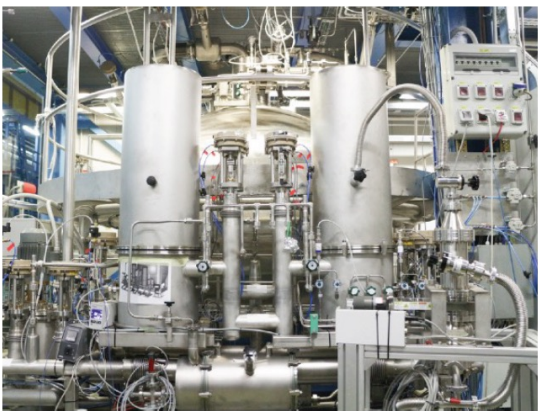
LXe purification system (5 L/min LXe, faster cleaning; 2500 slpm) for XENONnT
