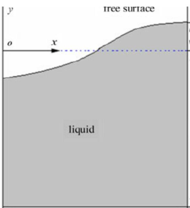
$$\frac{\partial \varphi}{\partial t} + \frac{1}{2} |\nabla \varphi|^2 + \frac{1}{\rho} p + gy = \text{const.}$$
