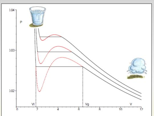
FIG. 2. Maxwell's equal area law. The 'oscillating' (dashed) part of the isotherm  $T < T_c$  is replaced by an isobar, such that the areas above and below the isobar are equal one another.
