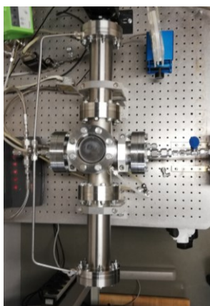
Figure: Left panel: Reactor for laser pyrolysis of carbon dots; Right panel: schematic representation of different precursors used to obtain carbon dots and their subsequent deployment on P25 nanoparticles.
